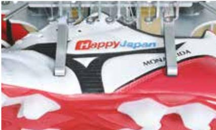
Telaio scarpa - Shoe Clamp (60x100mm)
